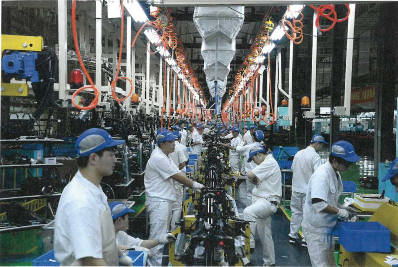
Chinese factory workers assemble motorcycles on the assembly line at the plant of Sundiro Honda Motorcycle Co., Ltd. in Taicang City, China. (CYNTHIA LEE/ALAMY)
